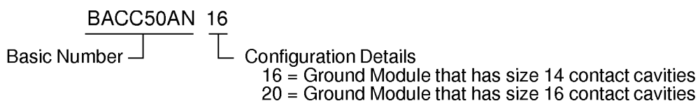
BACC50AN ENVIRONMENTALLY SEALED GROUND MODULE PART NUMBER STRUCTURE Figure 3
