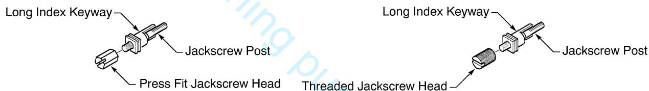
OBSOLETE JACKSCREW ASSEMBLY Figure 3
