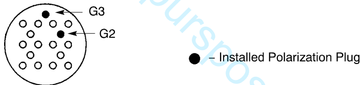
10-60540-1 AND 10-60540-6 RELAY SOCKET POLARIZATION - KEY G1 Figure 7
