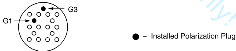
10-60540-2 RELAY SOCKET POLARIZATION - KEY G2 Figure 8
