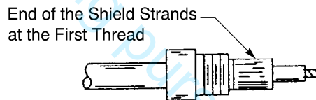
TERMINATION OF THE INNER SHIELD
